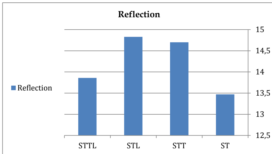
Figure 2. Values of reflection on the visible spectrum; (ST) standard sample; (STT) thermal aging; (STL) light aging; (STTL) after light and thermal aging
