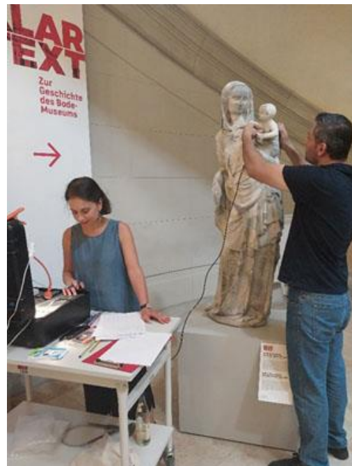
Figure 3. A photograph of performing ultrasonic velocity measurements on the sculpture of "Standing Mary with child" in Bode Museum.
