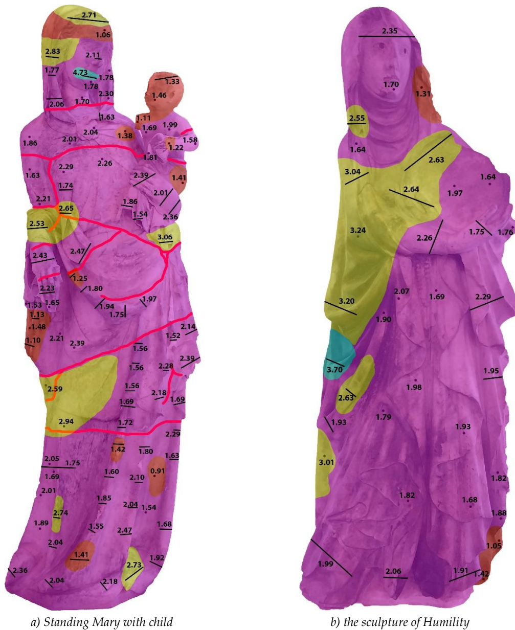
Figure 4. Mapping the damage classes of the sculptures based on ultrasonic velocity measurements and the adopted classification system (Table 2). The red lines indicate visible breaks and cracks, while the black lines and dots indicate the directions of ultrasonic measurement; the dots refer to front-back vertical directions.
